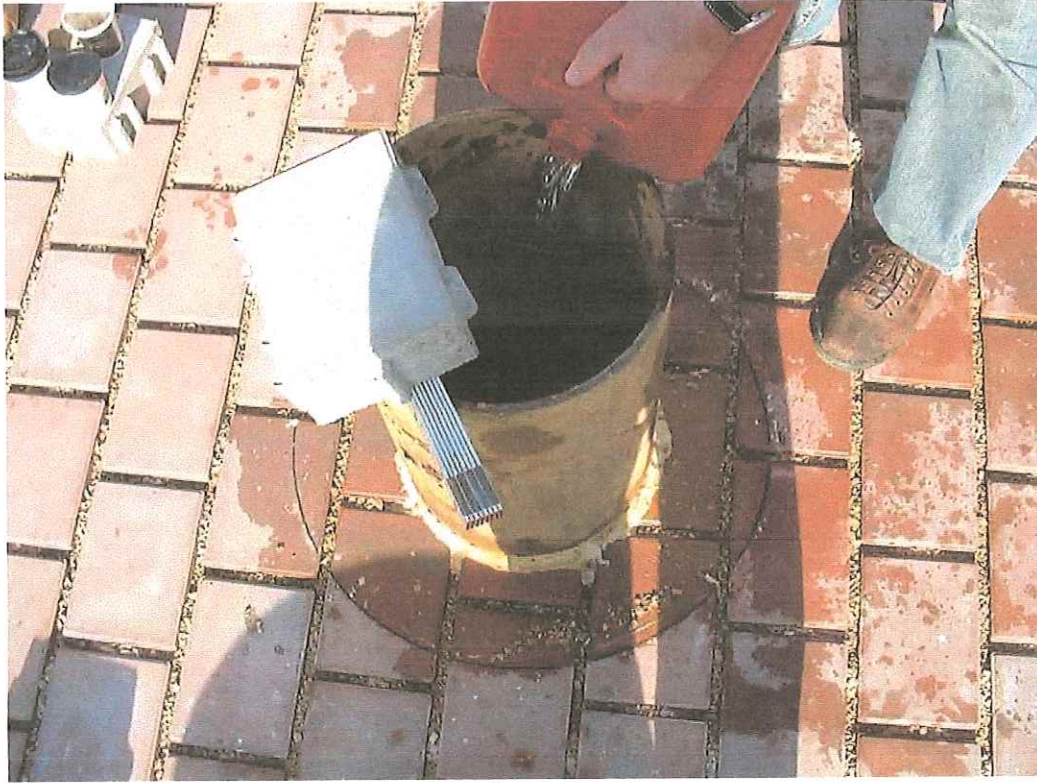
Single-ring placement for surface inundation test
