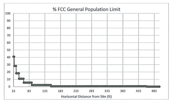
$Figure - 2 - calculated \ cumulative \ exposure \ level \ surrounding \ the \ proposed \ telecommunications \ facility \ expressed \ in \ percentage \ of \ the \ applicable \ FCC \ standard - antenna \ centerline \ level$
