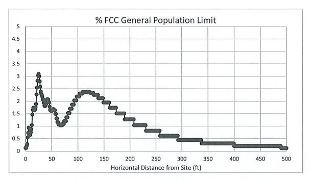
Figure-1 – calculated cumulative exposure level surrounding the proposed telecommunications facility expressed in percentage of the applicable FCC standard – ground level
