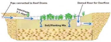
Source: Pennsylvania Stormwater BMP Manual (2006)
